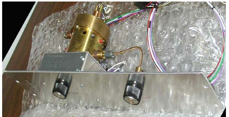
Phil Theis, K3TUF goes over some of the finer points of his water cooled 1296 amplifier
