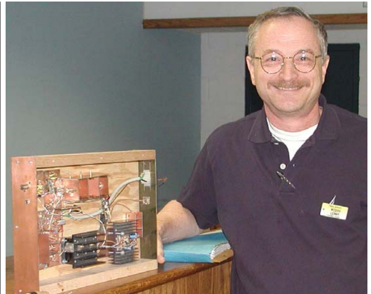
Lenny Wintfeld, W2BVH, gave us a tour of his zero budget, handcrafted modular construction 2 meter transverter
